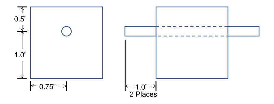
Cut (4) blocks 1.5" x 1.5". Drill and Install 5/16" dowels as shown above.
